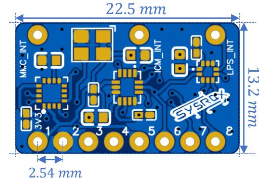
1. Sensors used are Invensense ICM42688-p, Memsic MMC5983MA and ST LPS22HB
